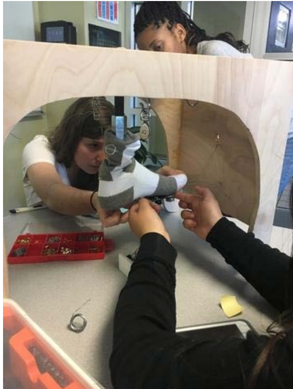
Figure 1 - The testing simulator being adjusted to fit the Lasso Compression Sock
